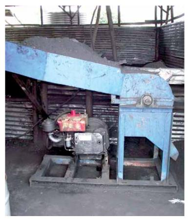
Mill for grinding cassava flour which is used as a dust mill to obtain green charcoal dust. Uganda.
