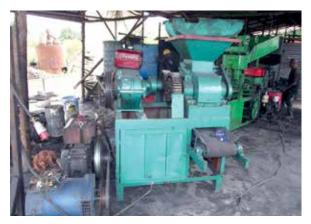
Machine, made in Uganda, which produces more than one tonne of green charcoal per hour.
