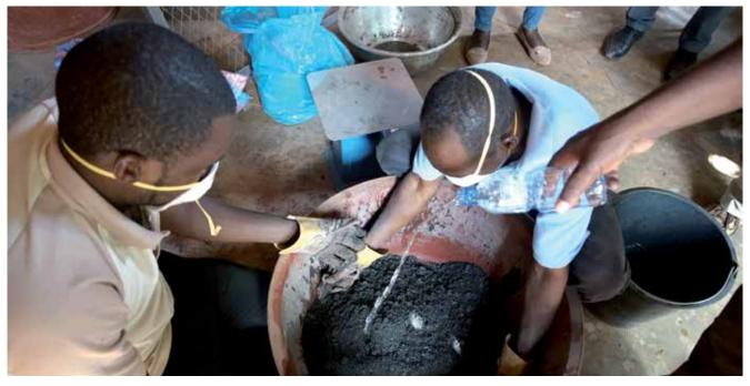
Added binder to powder after carbonization and grinding. Burkina Faso.
