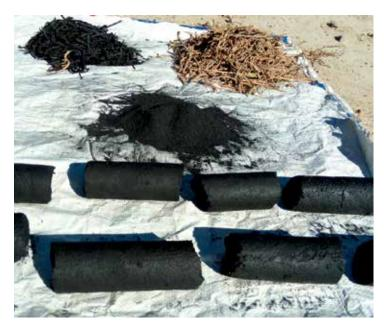
Raw materials (stems and rosemary leaves), carbonization product (dust), powder obtained after grinding and compressed and dried briquettes. Morocco.
